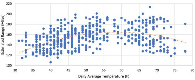
**Figure 10 notes:** Estimated vehicle range was calculated based off the %SOC per mile for each trip. The values represent the total estimated range if the bus is operated from 100% to 20% SOC.
