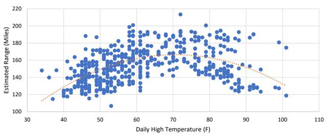
**Figure 11 notes:** Estimated vehicle range was calculated based off the %SOC per mile for each trip. The values represent the total estimated range if the bus is operated from 100% to 20% SOC.
