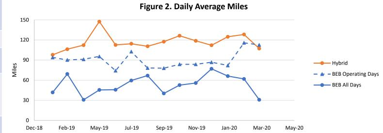
**Figure 2 notes:** The "Hybrid" and "BEB All Days" data series show the total monthly miles averaged over the total number of days per month and buses in the fleet, regardless of whether a bus was put into service. The "BEB Operating Days" series shows the total monthly BEB miles averaged over the days the bus was in service.
