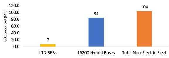
**Figure 14 notes:** Comparison of estimated CO2 emissions from various propulsion types during the pilot deployment period for the BEBs.
