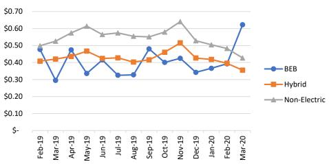
**Figure 3 notes:** Fuel costs per mile for the 16100 series BEB fleet, 16200 series hybrid fleet, and LTD's entire non-electric fleet are shown. Non-electric fleet fuel costs per mile fluctuate with changing diesel costs.
