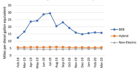
**Figure 4 notes:** Fuel economy for the 16100 series BEB fleet (miles per diesel gallon equivalent), 16200 series hybrid fleet (in miles per gallon), and non-electric fleet (in miles per gallon) are shown. BEB fuel economy increases in warmer months when the diesel heater is not utilized. Hybrid and non-electric fuel economies remain relatively constant.
