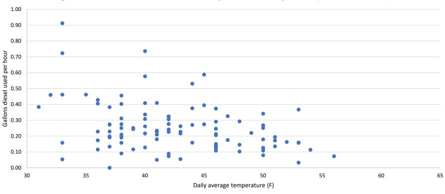
Figure 12. Gallons of diesel used/hour of operation vs. Temperature (2/3/19 - 3/18/20)
