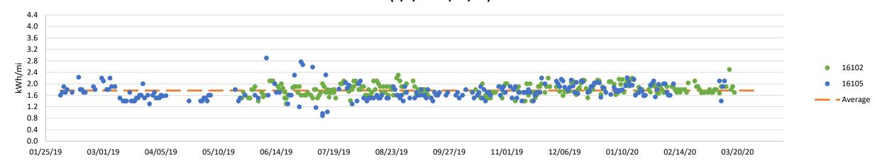
Figure 5 notes: Daily energy consumption (kWh/mi) by bus is shown, along with the overall average. HVAC consumption, driver style, and route conditions can impact energy efficiency.
