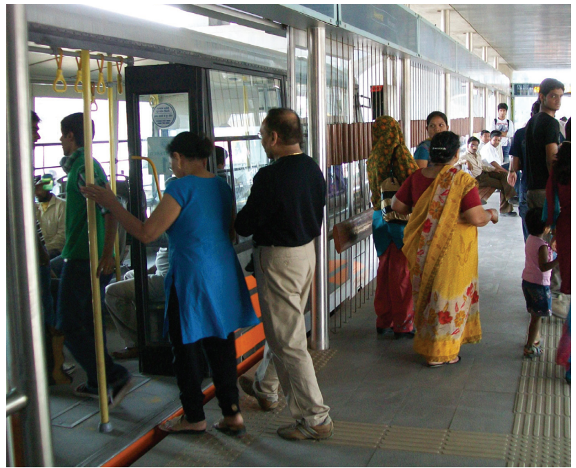
Passengers on Janmarg—Ahmedabad, India's new BRT—step directly from the platform onto the bus. Photo: ITDP
