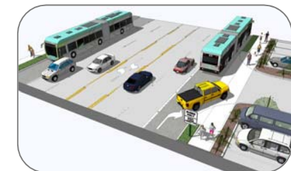
Business Access and Transitway Lane (BAT Lane)
