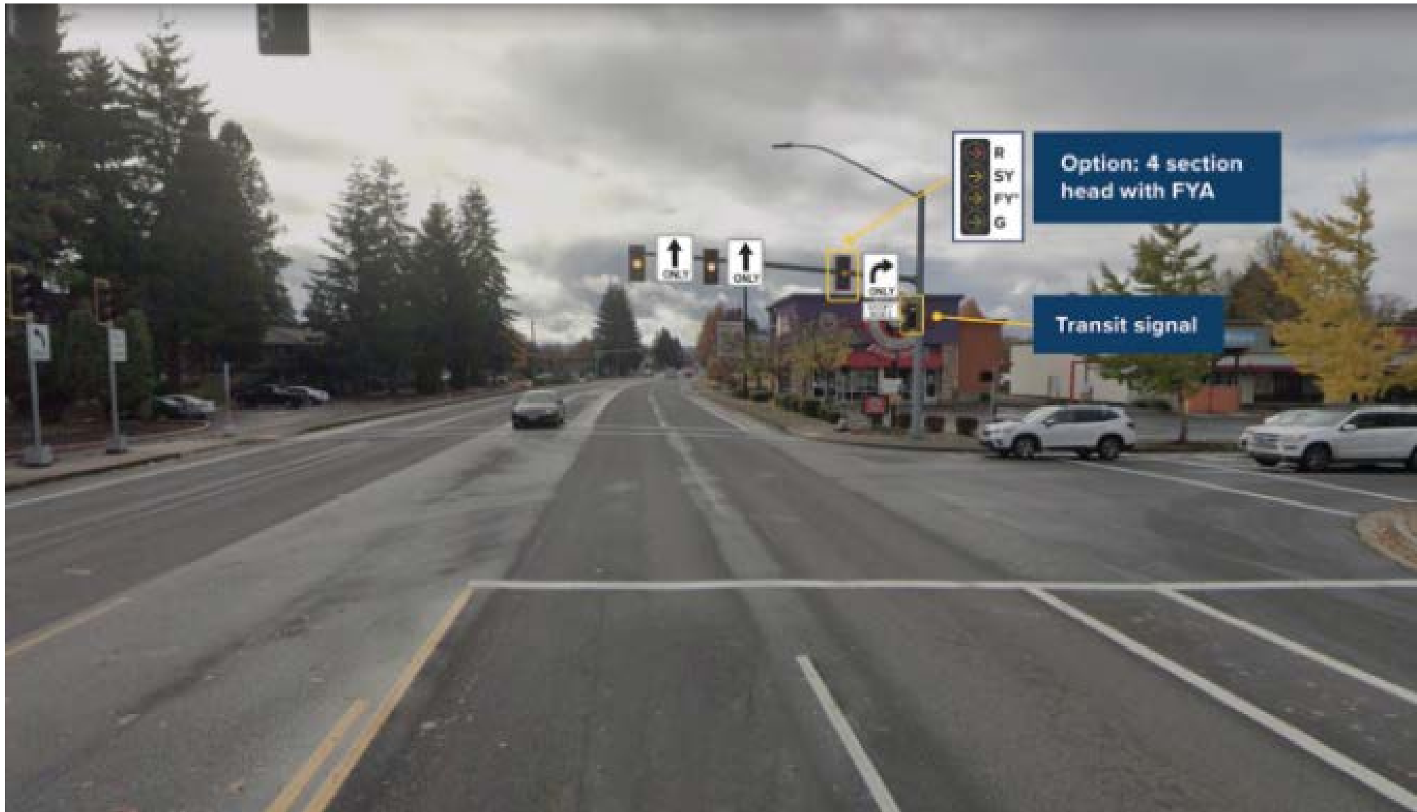
EXAMPLE SIGNALIZED INTERSECTION TREATMENT INSTALLATION (APPLIES TO QUEUE JUMP AS SHOWN OR THROUGH BAT LANE)
